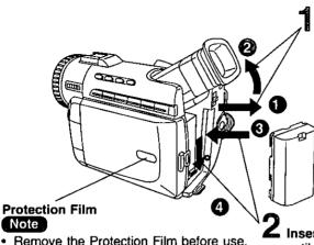
Slide the Viewfinder backward to its fully expanded position and then tilt it upward.
