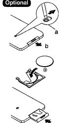
Insert a slender pointed object, such as the tip of a ball-point pen into the slot so that it fits into the hole (as shown a). Then, while sliding to the right, pull the Battery Tray out with your fingernail.
