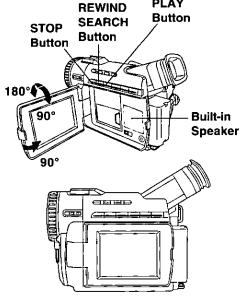
You can place the Palmcorder on a table, etc. for viewing. Rotate the LCD Monitor 180° and swing it up against the Palmcorder body as shown.
