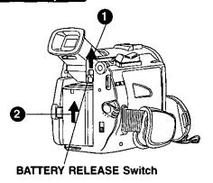
Slide the Battery upward while sliding the <u>BATTERY RELEASE</u> to **remove the Battery** (page 12).
