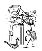
Thread the strap ends through the Strap Attachment Rings.
